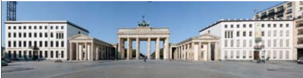
Flat projection (140°, horizontal field of view, straight lines, wide-angle distortion at the picture border)
