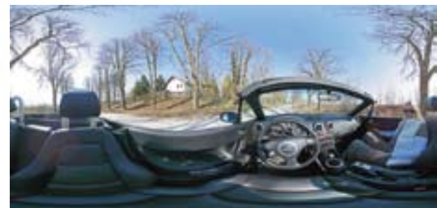
Spherical projection with 360° horizontal and 180° vertical picture field of view
